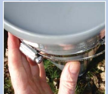
Hold down any excess band while finally tightening.
