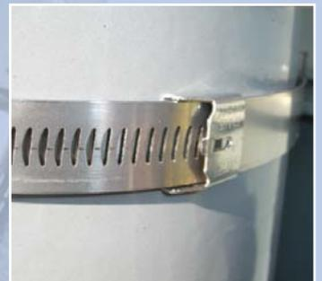
Push any excess band through the buckle for a safe, tidy job.
